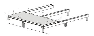
Insert a reinforced beam into the recessed edge of the first panel on the side that the second panel will attach to.
