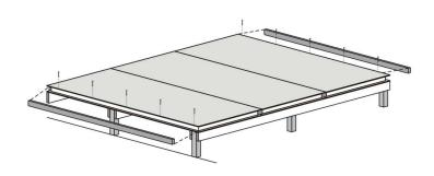
After completing the deck, flash along the perimeter with suitable material.
