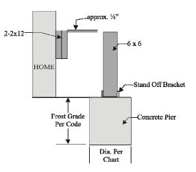
Level and secure 2x12 beams to both sides of the posts running parallel to the home. The beams should be mounted even with the top edge of the 2x12 ledger boards secured to the home. It is important that the beams be above the top of the posts.
