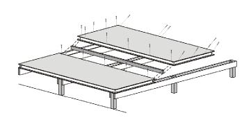
Once all the panels are installed, insert a reinforced beam along both sides of the deck. If the system has been ordered to accommodate lumber at the end of the panels, there will be a recess to insert 2x6 lumber into the end of the panels.
