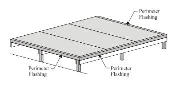
\*Please note that the supplied reinforced beams are treated with ACQ and can damage metal flashing. Take care to use a barrier between the flashing and the end of the reinforced beams.
